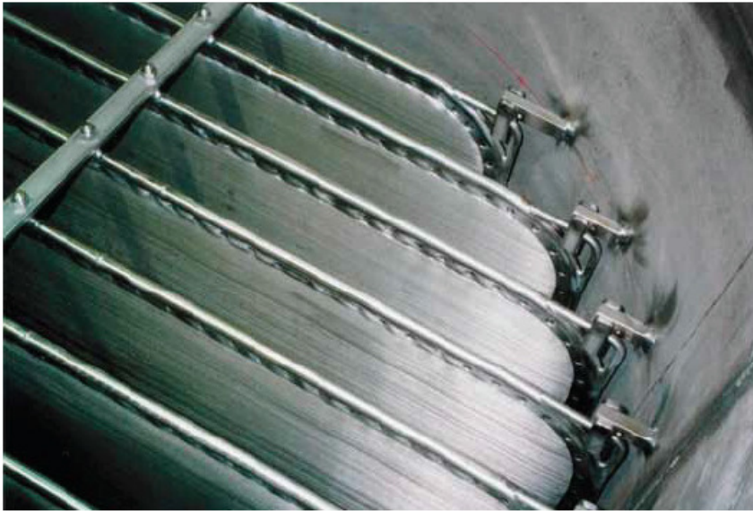
Figure 3: Filter Plates Interior View
